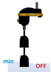
Low level stops the pump
