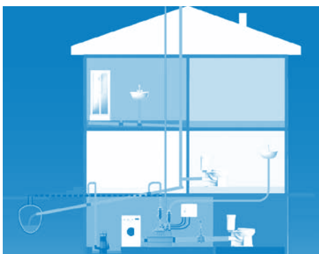
Figure 1: Example of installation with submersible pump:
